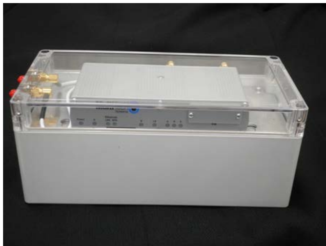
Figure 6-1 Embertec Savings Verification System (SVS) Data Logging Device
