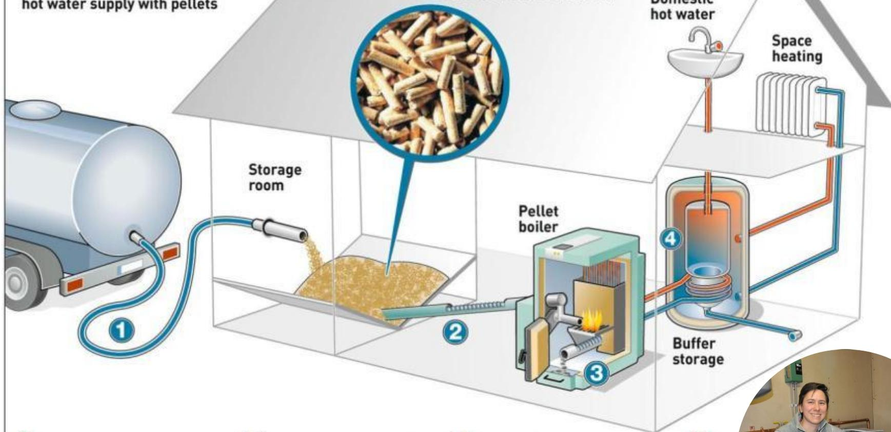
**1** Once or twice a year the pellets are delivered by a silo tanker. A loaded storage room of 4.5 m<sup>2</sup> is enough to keep a single-family house warm for one year.
