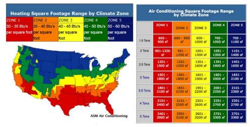
Figure 1: Examples of Simplified Sizing Guidance
