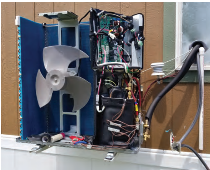
Figure 2-34. System F ODU with shrouds removed, thermocouples and pressure gauges installed
