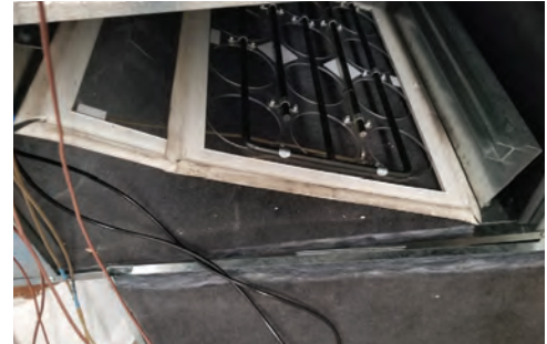
Figure 2-37. Ducted HP flow plate in filter slot (system A and B)
