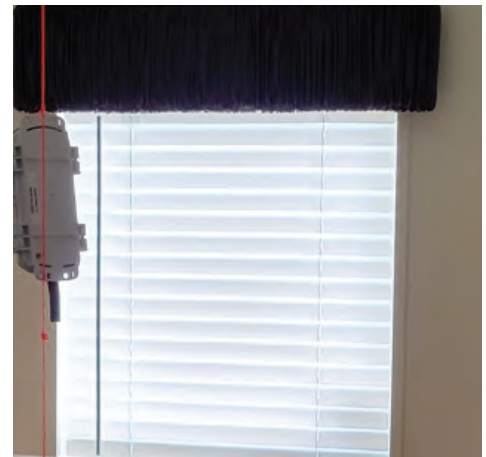
Figure 2-45. “BR2” wireless temperature and humidity sensor
