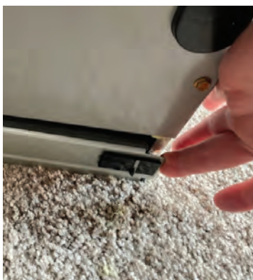
Figure 2-14. Broken latch on filter case
