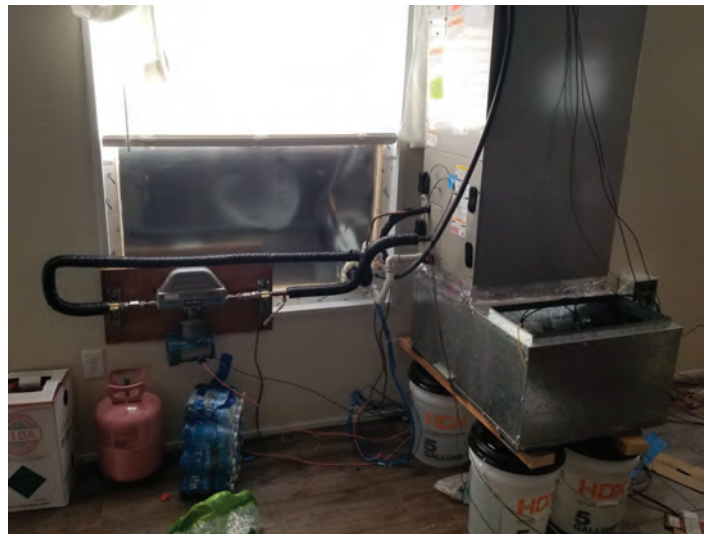
Figure 2-17. System A indoor unit with mass flow sensor
