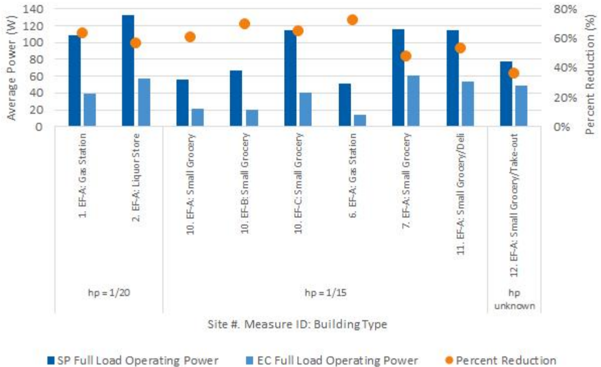
Figure 39. Unit Comparison – Average Pre/Post EF Motor Operating Power
