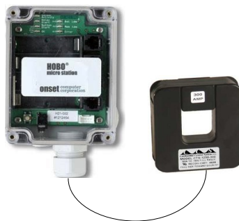
Figure B-2: Air Handler Logging Equipment
